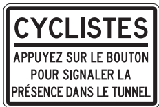
ID-15 CYCLIST PUSHBUTTON - TUNNEL (90x60)
